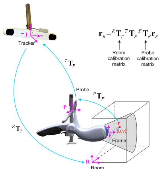
Figure 2. Schematic diagram illustrating coordinate transformations for calibration
