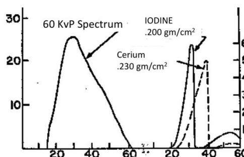
Figure 3. Formation of quasi-monoenergetic beams using filtration.
