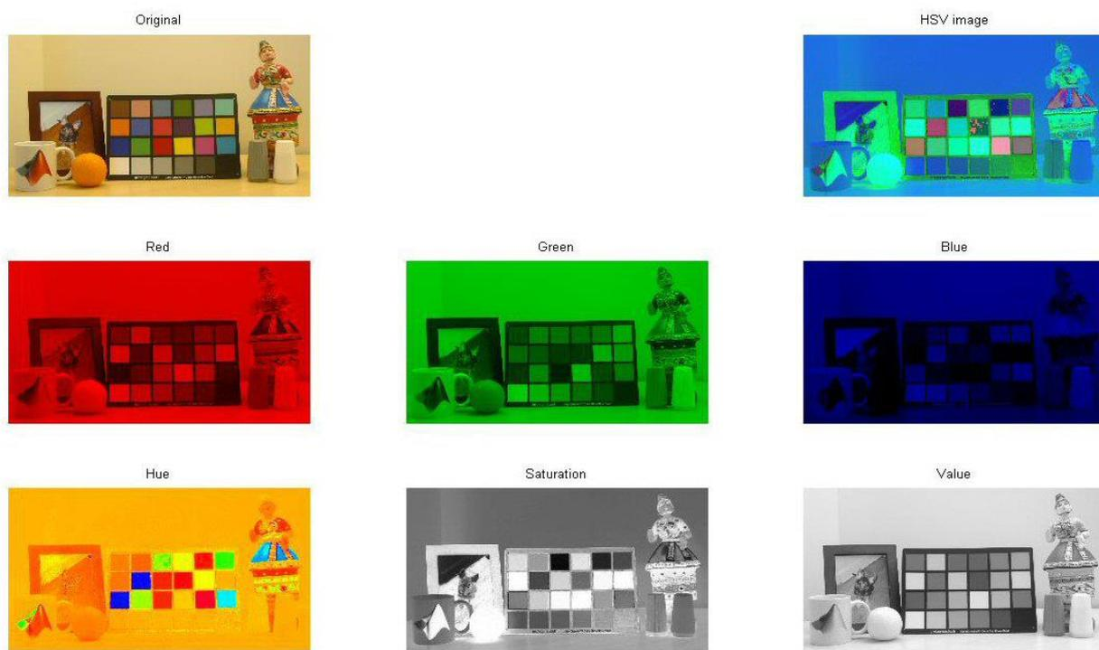
Figure 4. Illustration of the use of MatLab for decomposition of colour image – original image is decomposed to RGB and HSV (image courtesy to Dr A De Stefano).
