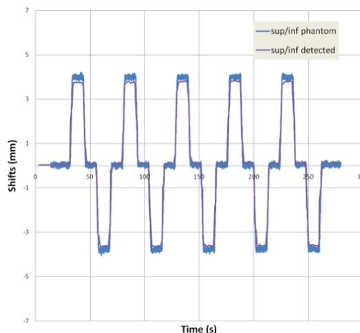
Figure 11. Comparison of programmed versus calculated motion in S/I directions
