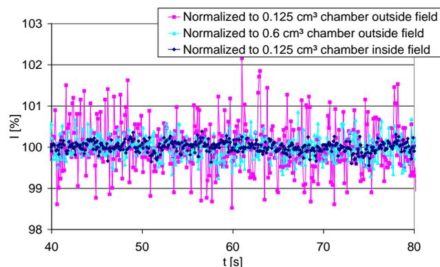
Figure 3. Signal of a 0.125 cm<sup>3</sup> chamber in a 4x4 cm<sup>2</sup> field at roughly 1.5 Gy/min, at 10 cm depth in water. The integration time for each data point is 100 ms. For this measurement, a 0.125 cm<sup>3</sup> reference detector has been placed inside the field (blue diamonds) and 3 cm outside the field (magenta squares). For comparison, the result when referencing to a 0.6 cm<sup>3</sup> Farmer chamber, located outside the field, is also displayed (cyan triangles).
