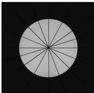
Figure 9. Line profiles for 16 directions ( $0^\circ$  (horizontal),  $11^\circ$ ,  $23^\circ$ ,  $34^\circ$ ,  $45^\circ$ ,  $56^\circ$ ,  $68^\circ$ ,  $79^\circ$ ,  $90^\circ$  (vertical),  $101^\circ$ ,  $113^\circ$ ,  $124^\circ$ ,  $135^\circ$ ,  $146^\circ$ ,  $158^\circ$ ,  $169^\circ$ ) to compute geometric distortion and linearity.
