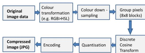
Figure 6. Simplified steps of the JPEG compression process
