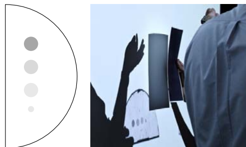
Fig. 1 (left) Semi-circular PMMA phantom with a number of disks of different graylevel representing a breast with lesions with different object contrasts. (right) The phantom is held up in front of two different “detectors” to show the difference in resulting image contrast.
