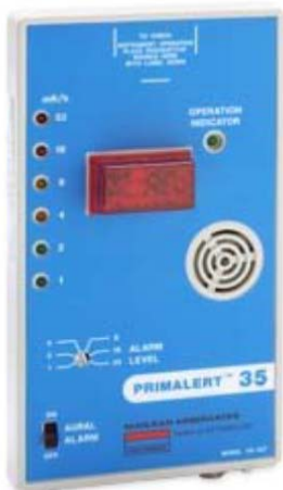
Figure 1. Sample image of a PrimAlert-35 G-M Radiation Detector
