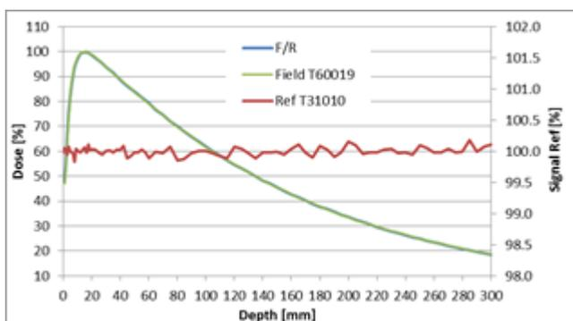
Figure 8: PDD measurements, 4 cm x 4 cm, field detector 60019, Varian Truebeam 6MV: a Semiflex 0.125 cm<sup>3</sup> used as reference chamber. Measuring time per data point 0.5s.
