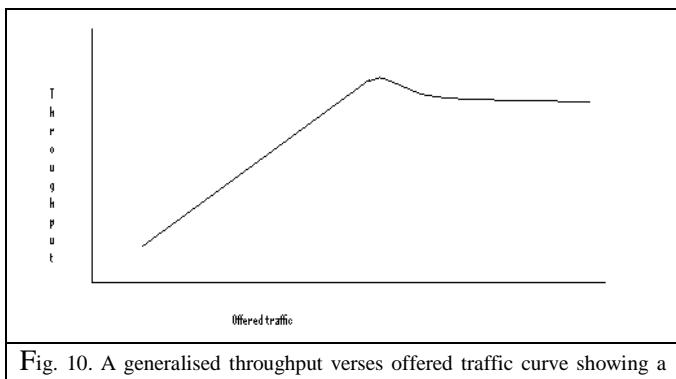
Fig. 10. A generalised throughput versus offered traffic curve showing a deterioration in performance when optimal levels are breached. – from TakTak et al [1]
