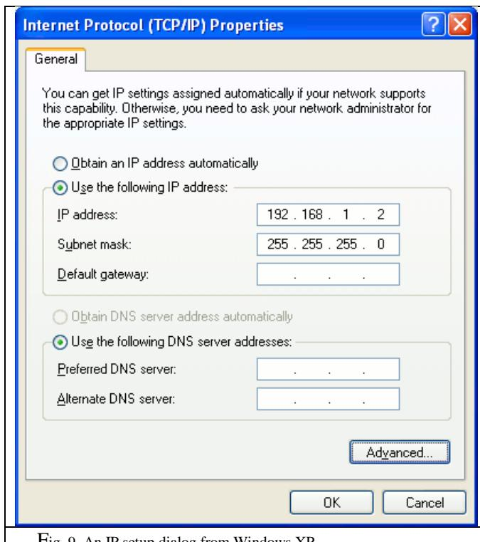
Fig. 9. An IP setup dialog from Windows XP
