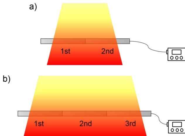
Fig. 4 Two- and three-step measurement process to measure CTDI by using the modified CTDI methodology
