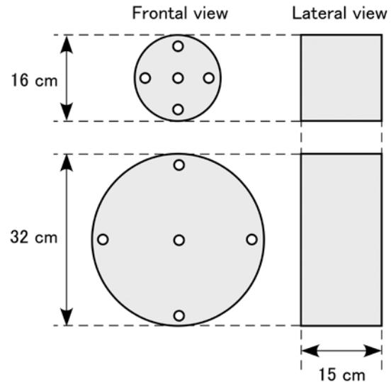
Fig. 1 Schematic of the polymethyl methacrylate phantoms
