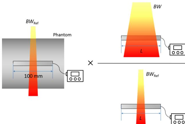
Fig. 3 Modified CTDI definition for an X-ray nominal beam width along the z-axis of >40 mm
