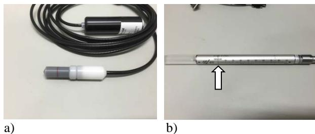
Fig. 5 Examples of small dosimeters for measuring accumulated dose at the midpoint of the scanning range: a) a Farmer-type 0.6-cm<sup>3</sup> ionization chamber (10X6-0.6CT; Radcal, Monrovia, CA, USA), b) a small solid-state detector (placed 3 cm from the end of the probe [white arrow]. CT Dose Profiler; RTI Group AB, Mölndal, Sweden)
