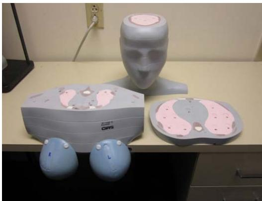
Fig. 6 An example of an anthropomorphic phantom (ATOM model 702; CIRS, Norfolk, VA, USA); it has holes for inserting small dosimeters
