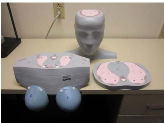
Fig. 6 An example of an anthropomorphic phantom (ATOM model 702; CIRIS, Norfolk, VA, USA); it has holes for inserting small dosimeters
