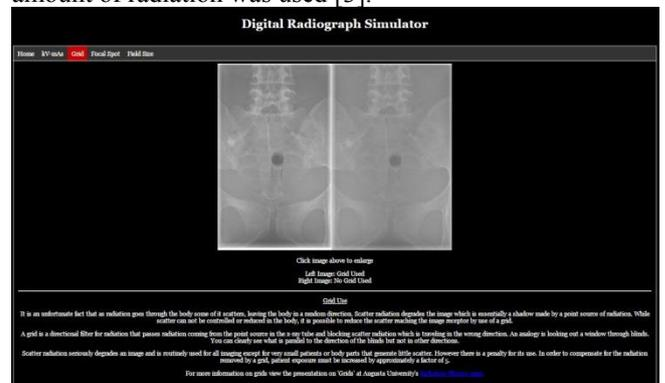
Fig 3. Comparison of Images Taken With and Without a Grid.
