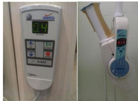
**Figure 1: On the left, a Gnatus machine with selectable times. On the right, an Astex machine with a preset menu**
