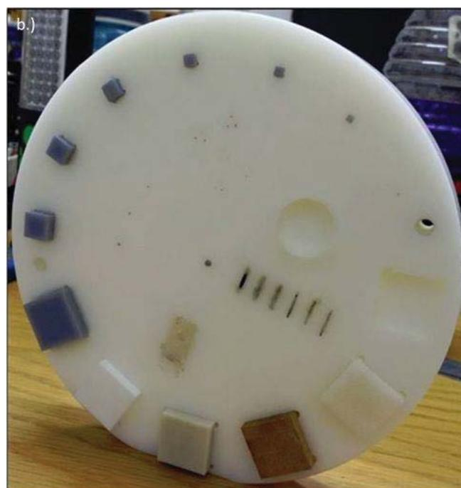
Fig. 1. A) The composition of the U-QA phantom showing the dimensions of the different inserts and the phantom. B) The bottom half of the U-QA phantom showing the different inserts in place.
