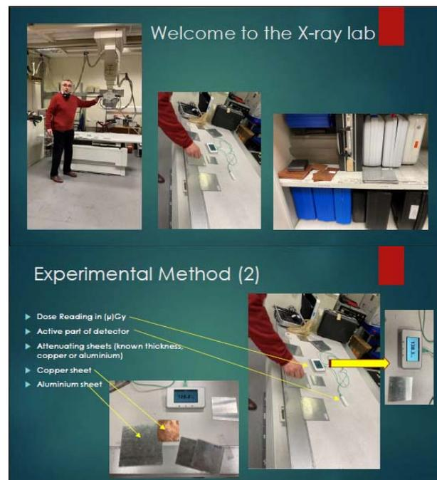
Fig. 2 Radiation Physics practicals – excerpt from the recorded material on Half Value Layer measurements.
