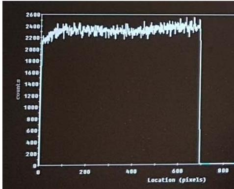
Fig. 4 Profile indicates problem of scanning mechanism.
