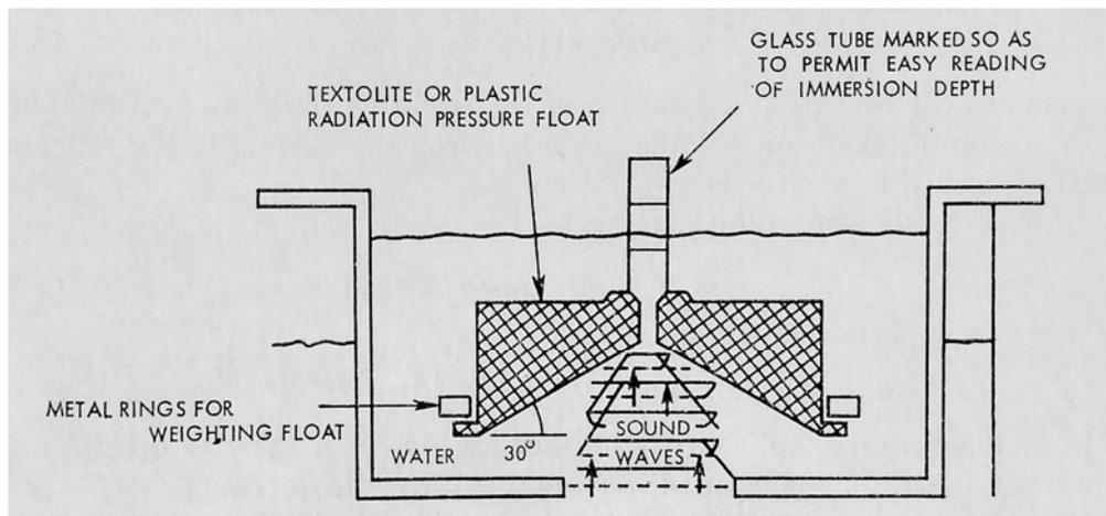
Fig 12. Henry's design for a power balance using a neutral buoyancy absorbing float target. 1957. [24] (©Iiffie Books Ltd)
