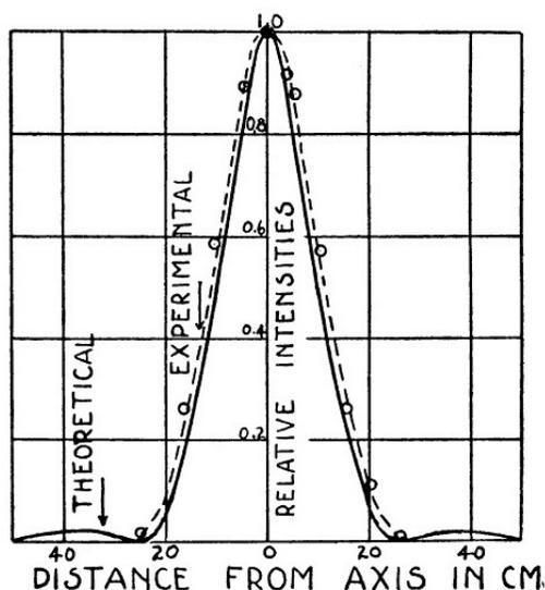
Fig 3. Measured and calculated intensity profiles using the torsion balance. Boyle 1928. [4]
