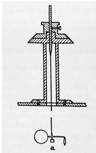
Fig 1. A torsion pendulum for the measurement of acoustic intensity.
