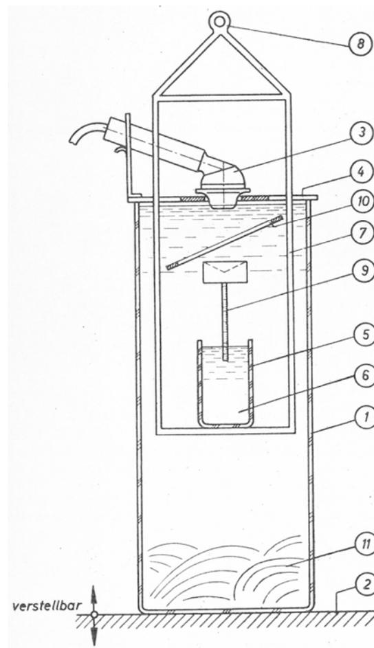
Fig 11. The PTB floating target power balance. 1952. The transducer 3, is centred over the streaming screen 10 above the buoyant target 9. The lower calibrated stem is lowered into carbon tetrachloride 6. Oberst & Rieckmann [22].
