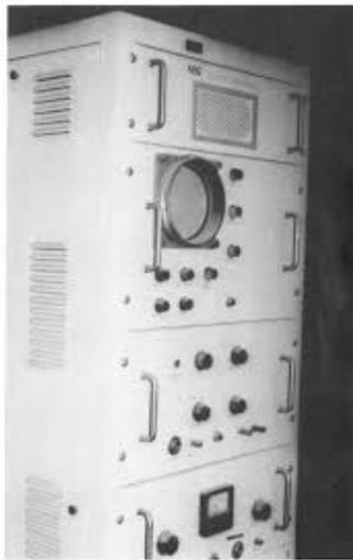
Fig. 4. First commercial Doppler ultrasound system; the 'Blood Rheograph' available in 1959 and developed by the Nippon Electric Company (Japan). Reproduced from *Ultrasound Med Biol*, Vol. no. 12, Kaneko Z, First steps in the development of the Doppler flowmeter, pp. 187-195, copyright Elsevier (1986).
