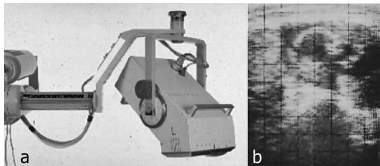
Fig. 33. a) The ‘Vidoson’ real-time water-bath scanner, was commercially introduced by Siemens Medical Systems, Germany, in 1965. As each of three transducers was rotated around the focal line of a parabolic mirror, its reflected beam was swept across the aperture, remaining parallel to the principal axis. b) An example of a single frame from an obstetric patient. Courtesy of the BMUS Historical Collection.
