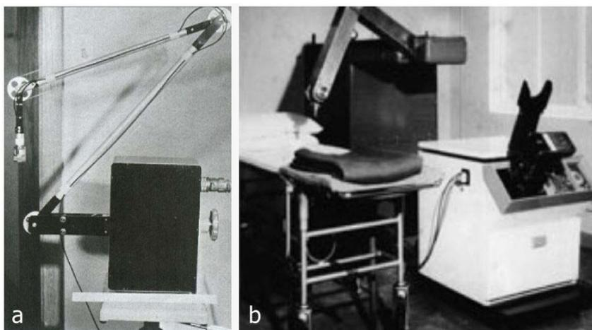
Fig. 31. a) The ‘Porta-Scan’ articulated-arm scanner designed in 1962, by engineers William Wright and Ralph Meyerdirk and commercially produced in 1963 by their own company, Physionic Engineering Inc., Colorado. b) A more sturdy articulated-arm scanner built by medical physicist Peter Wells, of Bristol General Hospital, UK around the same time as the Porta-scan. This was connected to an NE 4101 Diasonograph console, as shown. Photos courtesy of the BMUS Historical Collection.
