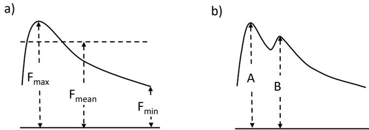
Fig. 8. Waveform indices. a) Measurements relevant to RI and PI. b) Measurements relevant to the A/B ratio.
