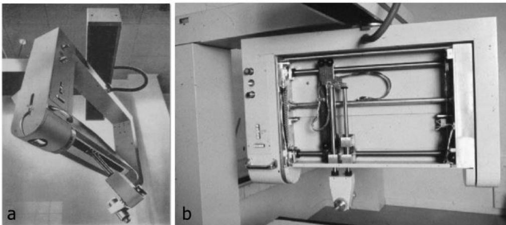
Fig. 23. a) Patient's view of the probe, the probe support box and the outer frame of the box, on an NE 4102. From Nuclear Enterprises Bulletin No. 64 [60]. b) View of the interior of the probe support box. The X and Y guide rails shown schematically in Figure 14 are prominent. Photo courtesy of the Design Council Slide Collection at Manchester Metropolitan University Special Collections.
