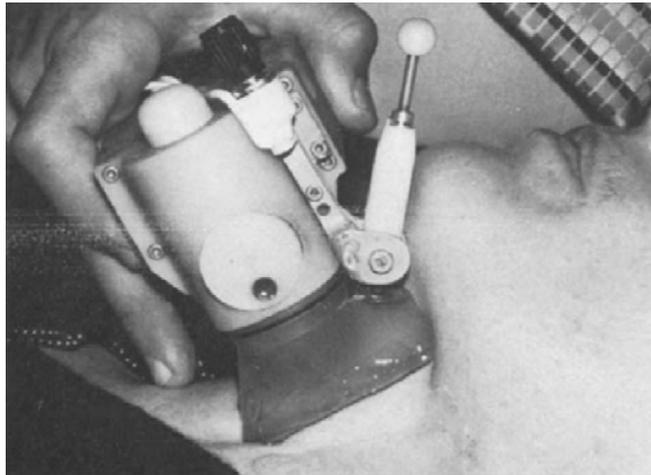
Fig. 10. 'Duplex III' transducer developed by Philips et al (1980). The offset Doppler probe is seen on the right of the transducer. Reproduced from *Ultrasound Med Biol*, Vol. no. 6; Phillips DJ, Powers JE, Eyer MK, Blackshear Jr WM, Bodily KC, Strandness Jr DE, Baker DW; Detection of peripheral vascular disease using the Duplex scanner III, pp. 205-218, copyright Elsevier (1980).
