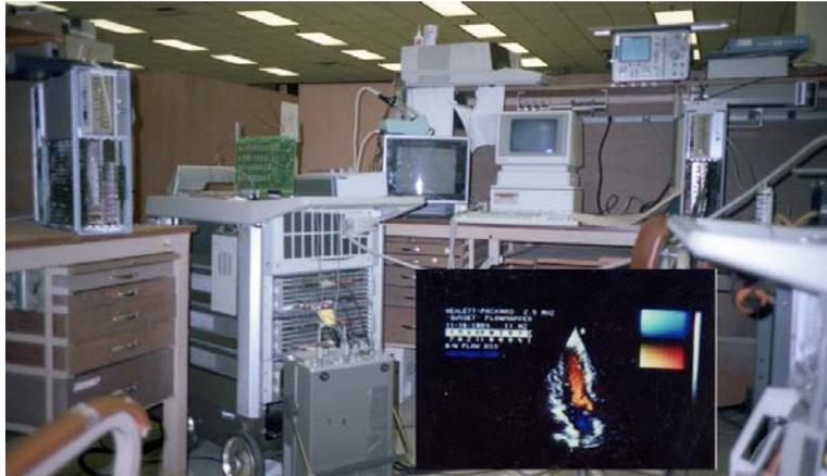
Fig. 12 First HP prototype color flow mapping system, Nov. 1984, Insert: color flow image. (Courtesy, Barry Hunt).
