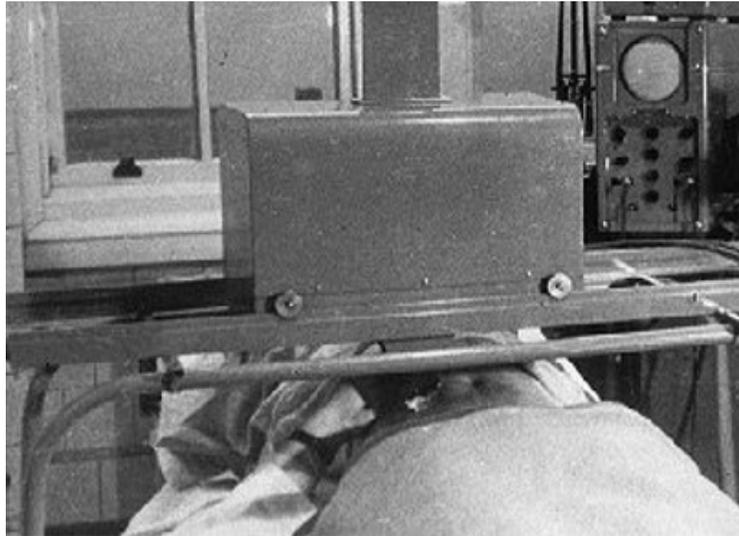
Fig. 7 Tom Brown’s bed-table scanner, c 1957. Note the restricted room for the operator’s forearm and hand (seen lower left). Photo courtesy of the BMUS Historical Collection
