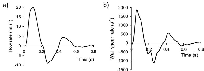
Fig. 13. Estimation of volumetric flow and wall shear stress (Blake et al. 2008 [164]).
