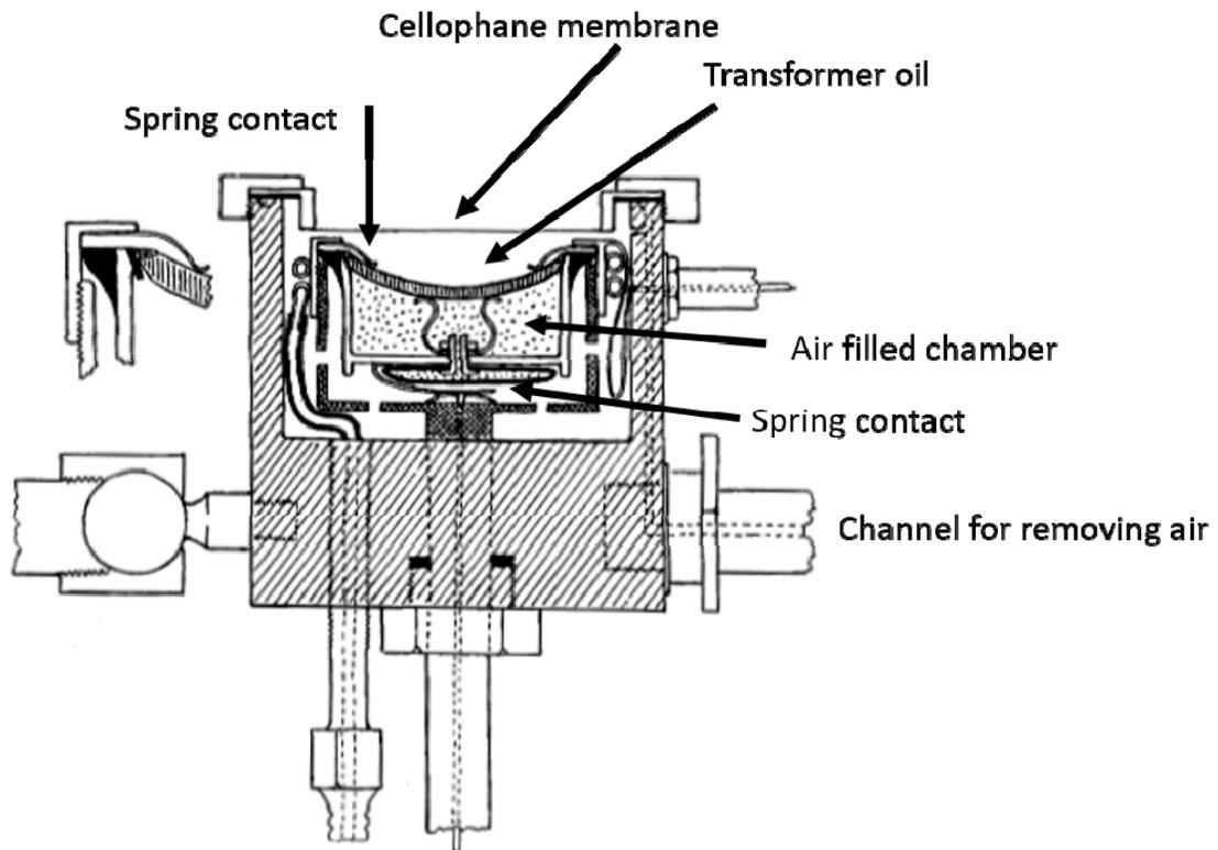
Fig. 3 Transducer mount used by Lynn et al (11).
