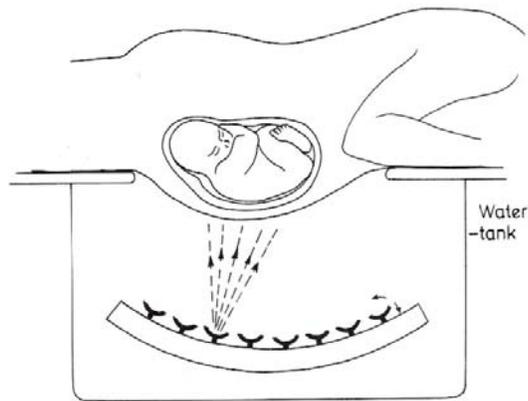
Fig. 5 Basic structure of the UI Octoson scanner.
