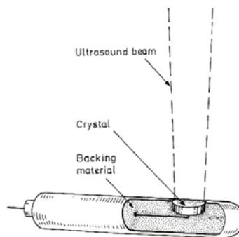
Fig. 12 Transducer for  $360^\circ$  radial invasive scanning.
