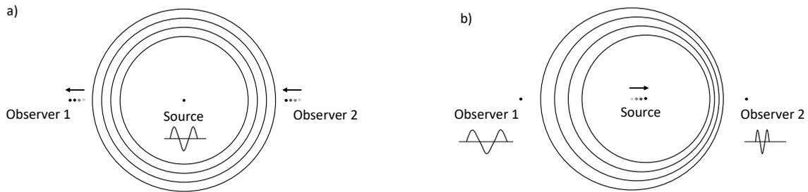
Fig. 1. Doppler effect; there is relative movement between the source and the 2 observers. a) Wave motion with respect to the source. The wave propagates symmetrically in all directions at a frequency  $f$ . b) Wave motion with respect to the observers. Wave propagation is asymmetric; there is contraction of the wave as perceived by Observer 2 who perceives a higher frequency ( $f_2 > f$ ); for Observer 1 there is dilation of the wave who perceives a lower frequency ( $f_1 < f$ ).
