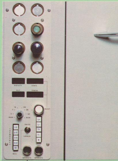
Probe storage—digital read-out of scanning frame position and angulation—stepping motor control—tuned amplifier frequency selector.
