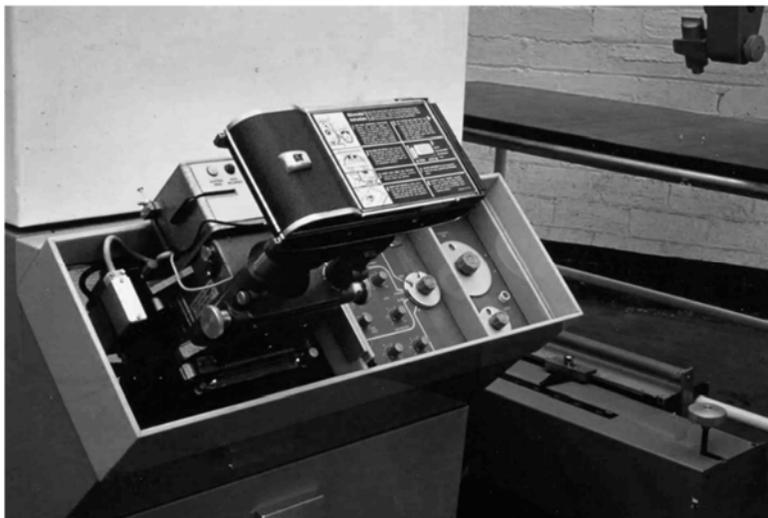
Figure 21. The controls on the console of the Smiths' Disonograph, with the three levels of control and Polaroid camera, designed by Dugald Cameron. Photo reproduced by the kind permission of Dugald Cameron
