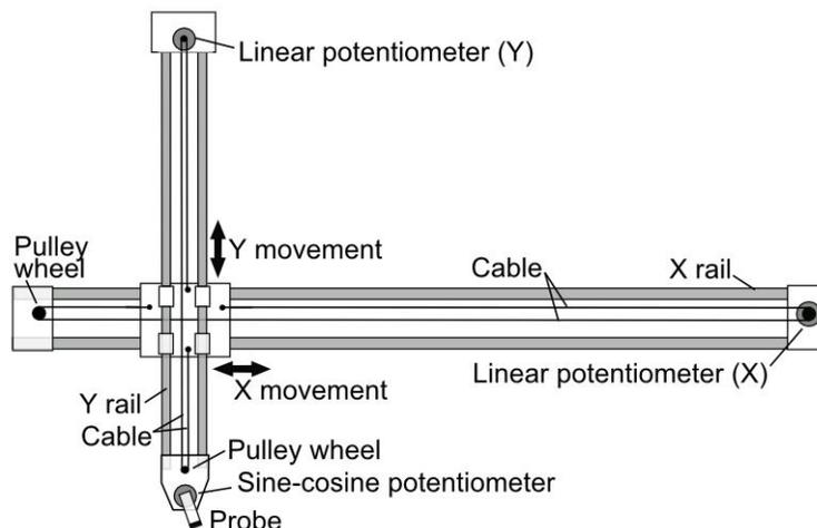
Fig. 14 Illustrating the principle of the system used to support and constrain the probe within the scan plane and to obtain the X,Y and angle coordinates of the probe relative to the scan plane.
