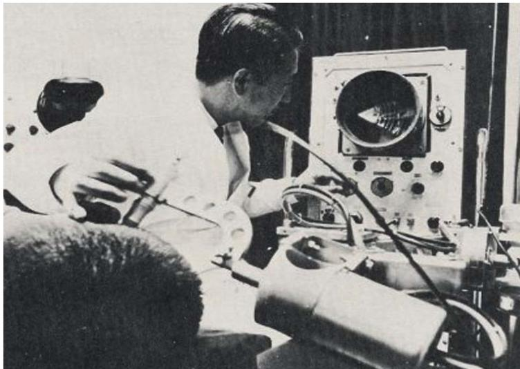
Fig. 30 The One-point Contact Sector Scanner of Kikuchi [83] being used by to scan a brain c 1957. It was also used successfully, later, in obstetrics and gynecology. Courtesy of the BMUS Historical Collection.
