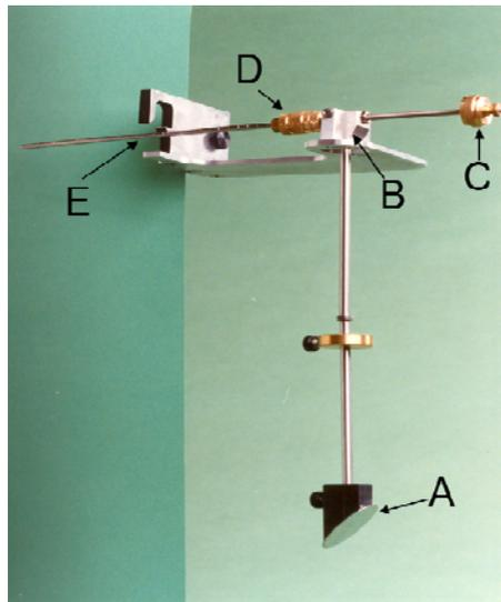
Fig. 6 Equilibrium balance for measuring radiation force
