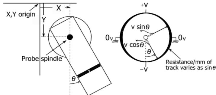
Fig. 9 Left: Measurement of probe angle  $\theta$  relative to the Y axis of the scan plane. Right: The 'cosine' wiper of the sine-cosine potentiometer is at the same angle as the principal axis of the probe.
