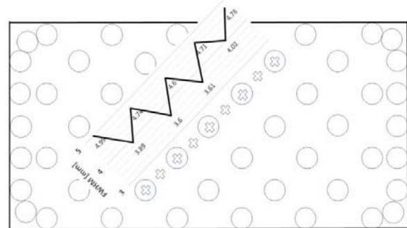
Fig. 6 Graphs of spatial resolution at 9 reference points marked with "x" in chess-board arrangement of PMT.
