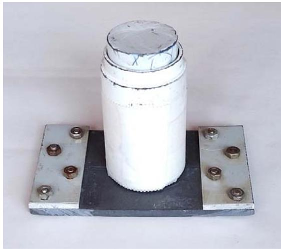
Fig. 1 Slit phantom with encapsulated source.
