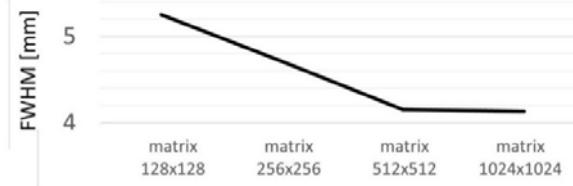
Fig. 3 Effect of pixel size on spatial resolution result
