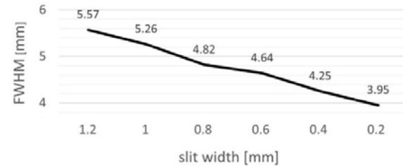
Fig. 2 Effect of slit width on spatial resolution result.
