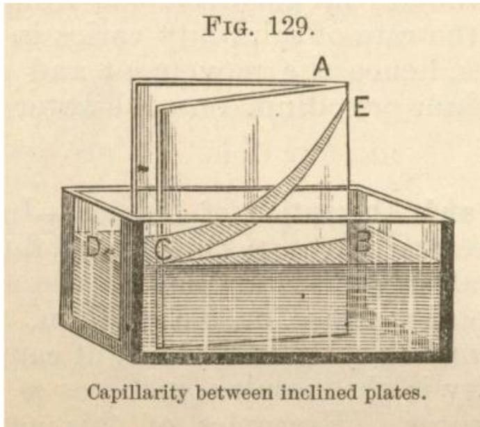
The apparatus shown in Fig. 129 was used to demonstrate capillary action that occurs between the surfaces of a solid and a liquid. Two glass plates are separated with a wedge shape as shown and placed in a tank of water. The water is pulled up by capillary action between the solid and liquid media. It is pulled to the greatest height where the glass plates are the closest.
