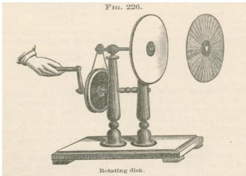
Newton's rotating disk shown in Fig. 226 is one method used to demonstrate the composition of light as a mixture of different colors. Disks divided into segments of various colors are mounted on the spinning apparatus. When they are spun at a high speed the composite color is observed. This would be white when the segments of the disk contain the spectrum of colors that are in white light.
