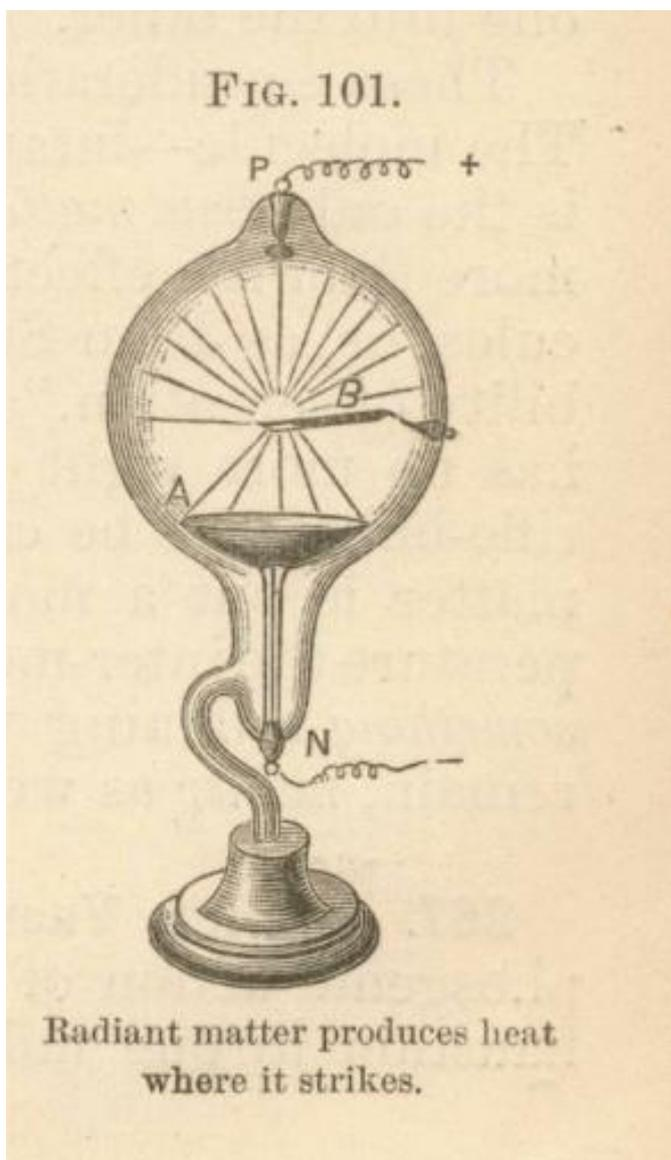
The tube shown in Fig. 101 was used to demonstrate that radiant matter produced heat when it was absorbed in a material. It contained a small platinum plate at the positive terminal (B) and a focused cup at the negative terminal as shown. When it is connected to an electrical source radiant matter is focused on the platinum plate heating which becomes red-hot. The heat radiates to the glass tube causing it to become warm.
