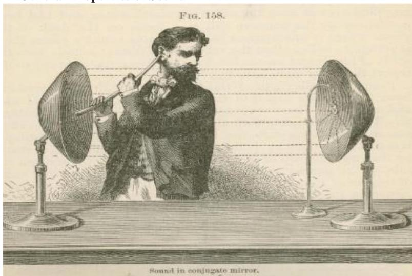
Figure 158 is a demonstration of the reflection of sound between two parabolic mirrors. A watch is placed at the focus of the mirror on the right. The sound is then reflected in parallel lines to the mirror on the left. It is then re-focused where it can be conducted to the ear as illustrated.
