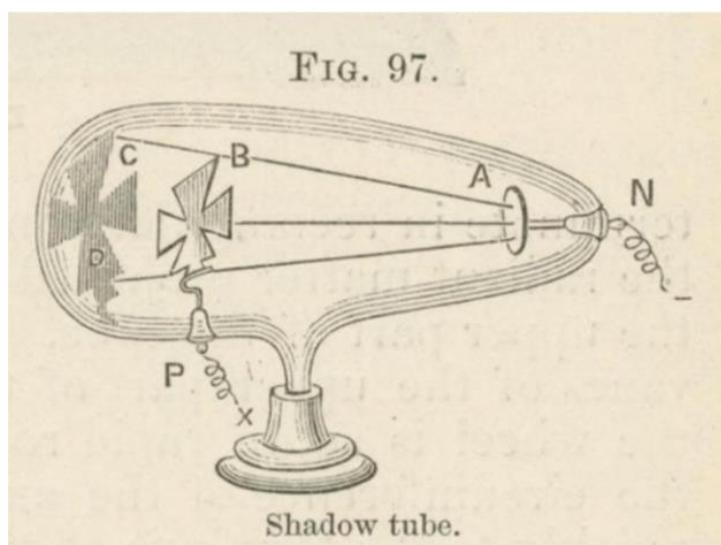
The tube shown in Fig. 97 was used to demonstrate that radiant matter traveled in straight lines and could cast a shadow. When the two electrodes in the tube were connected to a coil providing a high voltage the large end of the tube glowed where it was exposed to the radiant matter. The metal star mounted in the tube intercepted the radiant matter and cast a shadow.
