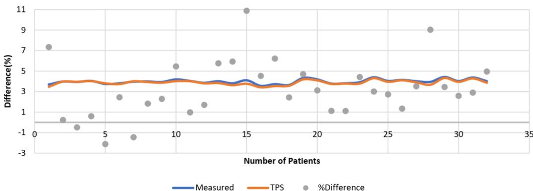
Figure 4: Agreement of the dose measured by an ionization chamber and TPS
