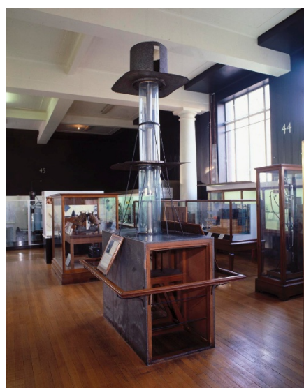
Fig 10. The accelerator tube of Cockcroft and Walton's accelerator on display in the Science Museum, London. The wooden observation chamber was closed by a curtain to provide a darkened space in which they could detect scintillations on a fluorescent screen.
