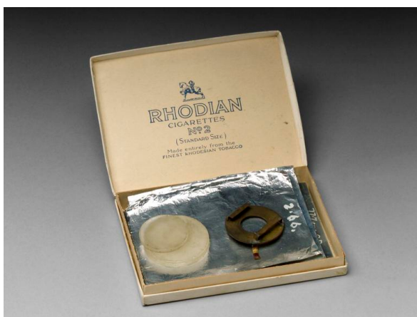
Fig. 4. Paraffin wax target, metal foils and foil holder which Chadwick used in his neutron experiments. This item is also on display in the London Science Museum
