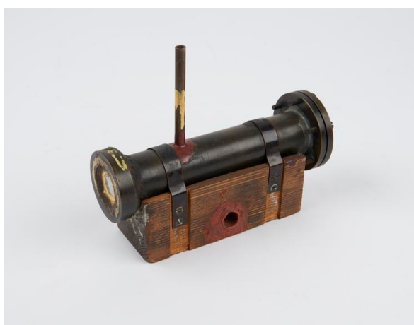
Fig. 3. The proportional counter Chadwick used to detect the recoil protons from the interaction of neutrons with the paraffin wax. The counter is on display in the Science Museum, London
