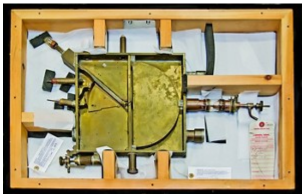
Fig. 7. Lawrence and Livingston's 11-inch cyclotron which produced an energy of 1.2 MeV.
