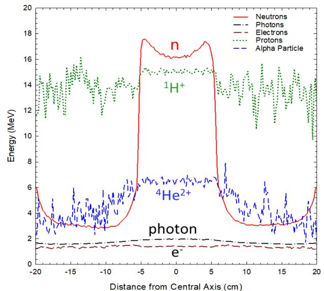
Fig. 26 Distribution of neutrons and secondary particles in the UW CNTS beam. (Reproduced from ref. 30.)
