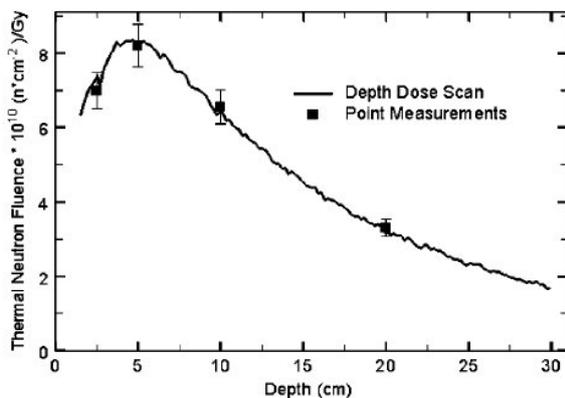
Fig. 31 Thermal neutron fluence as a function of depth in water measured in the WSU/KCC BNCFNT beam. (Reproduced from ref. 14.)
