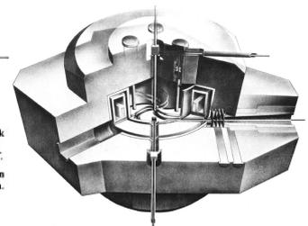
Fig. 8 Patent and cutaway view of the superconducting cyclotron for FNT at WSU/KCC. (Images courtesy of the author.)
