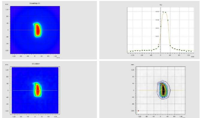
Fig.22 Representative MLC shape from segmental IMNRT delivery evaluated using a tissue-equivalent gas filled ion chamber array for IMNRT quality assurance at WSU/KCC. (Reproduced from ref. 23.)
