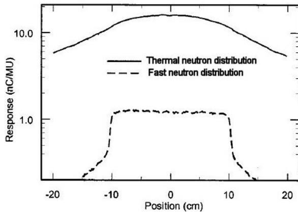
Fig. 30 Measured thermal neutron and fast neutron profiles in the WSU/KCC BNCFNT beam measured using ionization chambers with (thermal neutron) and without (fast neutron)  $^{10}\text{B}$  loading. (Image courtesy of the author.)
