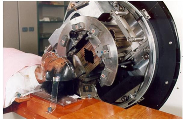
Fig. 7 Multi-blade trimmer for the iThemba fast neutron therapy facility. (Photo courtesy of Dan Jones.)
