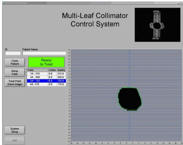
Fig. 18 WSU/KCC computer-controlled MLC system interface. (Image courtesy of the author.)
