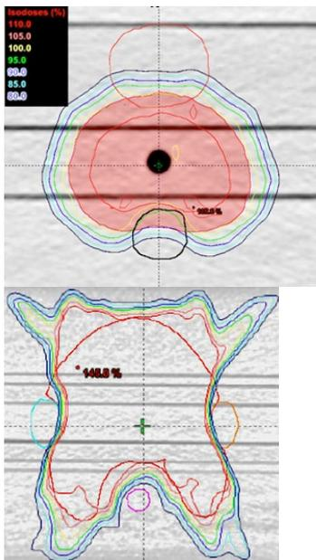
Fig. 21 Calculated dose distributions for the TG-119 mock prostate and head and neck cases during IMNRT commissioning at the WSU/KCC FNT facility. (Images courtesy of the author.)
