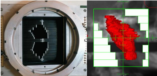
Fig. 5 UW CNTS MLC (left) along with MLC shape for representative radiotherapy target (right). (Reproduced from Wikipedia.)
