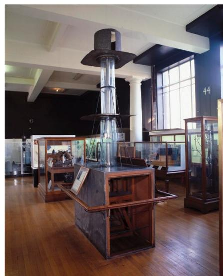
Fig 10. The accelerator tube of Cockcroft and Walton's accelerator on display in the Science Museum, London. The wooden observation chamber was closed by a curtain to provide a darkened space in which they could detect scintillations on a fluorescent screen.
