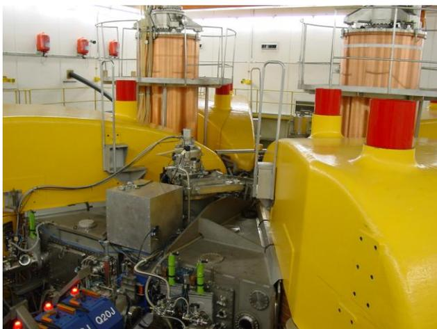
Fig. 10 Separated-sector cyclotron at iThemba Labs near Faure, South Africa. Yellow objects are the C-shaped bending magnets.
