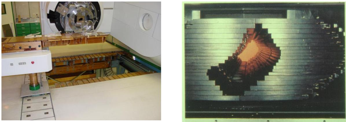
Fig. 28 (L) Multi-blade collimator at iThemba Labs. Note the retractable false floor to allow gantry rotation. The floor and patient positioner top were made of wood to reduce radioactivation. (R) Programmable multi-leaf collimator at UW. Reproduced from Scanditronix MC series cyclotrons brochure.
