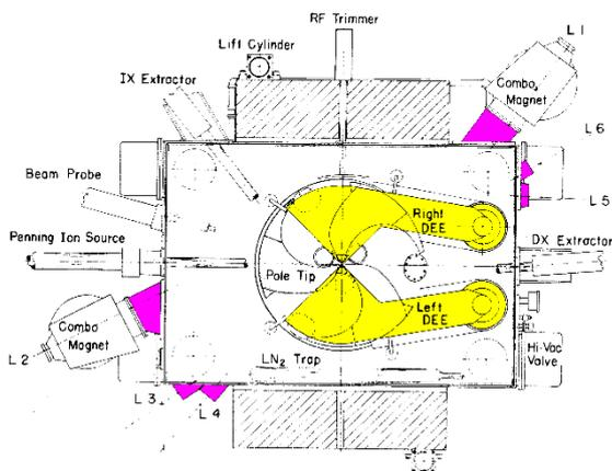
Fig. 7 Diagram of TCC cyclotron layout.
