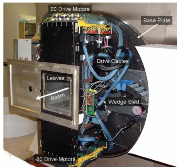
Fig. 17 The WSU/KCC MLC mounted on the gantry, shown here without the cover. (Reproduced from ref. 16.)
