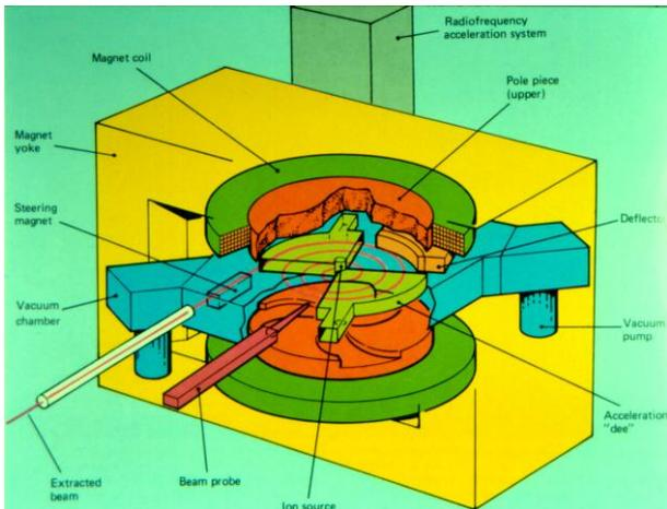
Fig. 9 Diagram of positive ion cyclotron produced by Scanditronix. Reproduced from Scanditronix MC series cyclotrons brochure.
