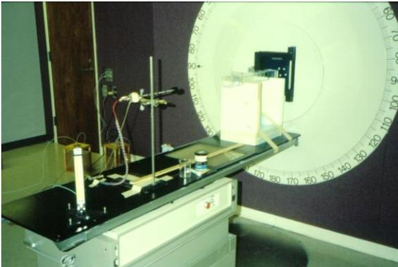
Fig. 30 Setup for measuring attenuation data used in deriving the neutron and photon spectrums. A variable but discrete thickness water column was used to provide narrow beam attenuation. Attenuation measurements were repeated with one chamber being sensitive to both neutrons and photons while a second chamber was sensitive primarily to photons.
