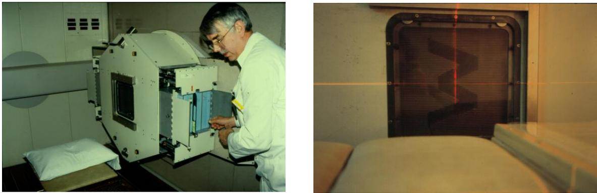
Fig. 27 Tungsten rod array for patient-specific collimation at WSU. (L) Richard Maughan inserting cut Styrofoam blocks used to move the rods into place. (R) A reverse beam's eye view of the tungsten rods after having been moved into place.
