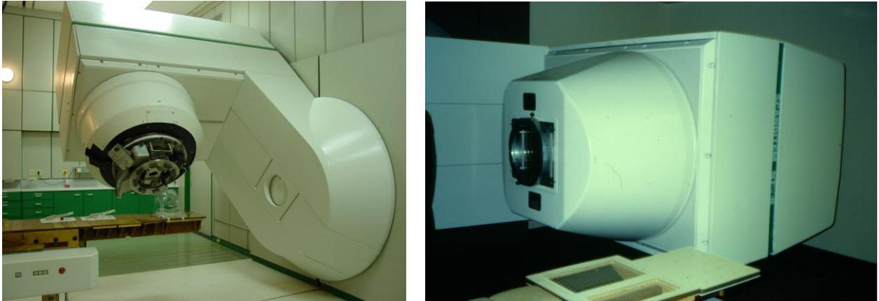
Fig. 14 Examples of fully rotating slewing ring gantries. (L) iThemba Labs. (R) University of Washington. For beams pointing upwards, floor panels would shift to the side allowing the radiation head to be rotated into a pit below the level of the false floor. The major difference between the two gantries is the shape of the collimator housing.
