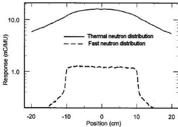
Fig. 30 Measured thermal neutron and fast neutron profiles in the WSU/KCC BNCFNT beam measured using ionization chambers with (thermal neutron) and without (fast neutron) <sup>10</sup>B loading. (Image courtesy of the author.)
