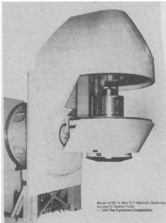
Fig. 2 Picture of gantry and opened radiation head for TCC based fusion source. Reprinted from Bloch et al. [6] with permission from IEEE.
