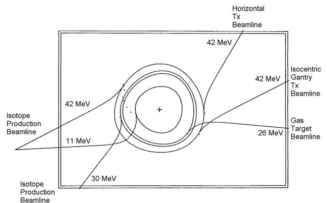
Fig. 8 Diagram showing stripping foils paced at different locations around the cyclotron to intercept different energy orbits and extract beam through one of five different extraction ports.
