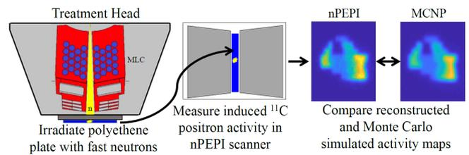
Fig. 25 Patient specific QA tool comparing MC calculated  $^{11}\text{C}$  decay maps with measured induced  $^{11}\text{C}$  activity using neutron positron emission portal imaging. (Image courtesy of Robert Stewart.)
