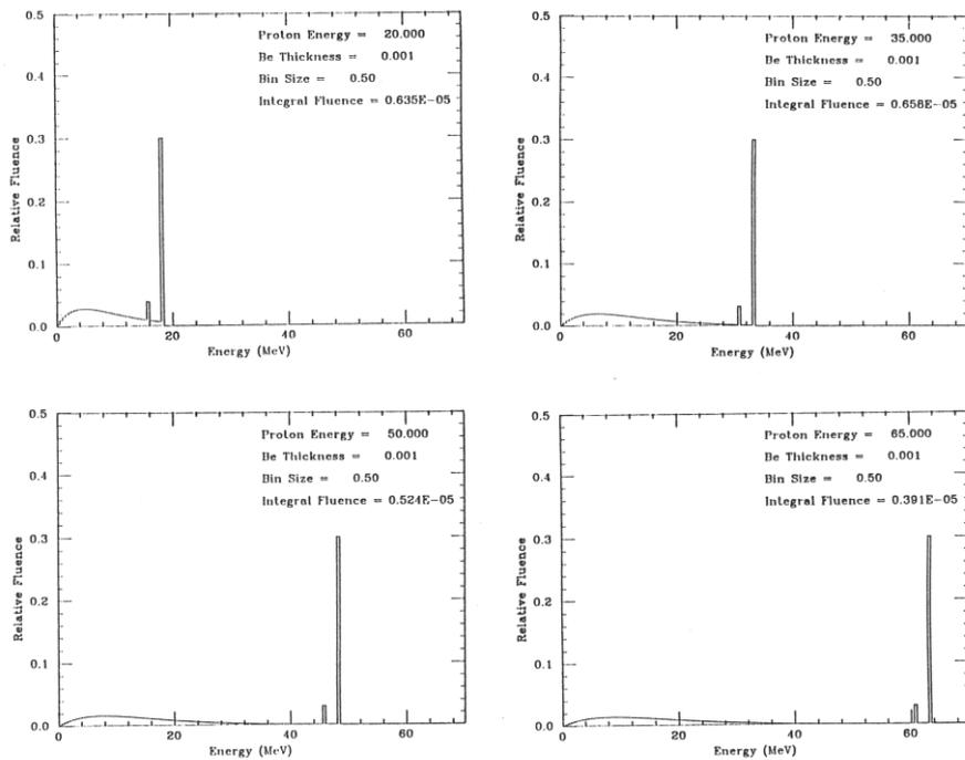
Fig. 18 Neutron production spectrum in the forward direction for different energy proton beams incident on a thin beryllium target. Reproduced from Moyers [12].
