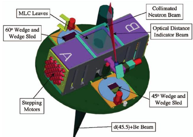
Fig. 16 Rendering of the high-resolution, computer-controlled MLC developed for the WSU/KCC FNT facility. (Reproduced from ref. 16.)
