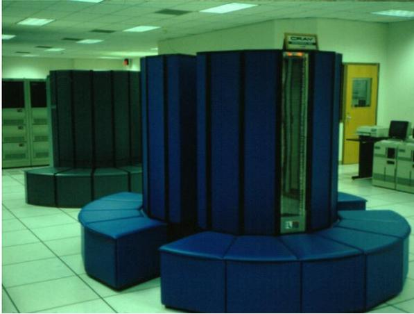
Fig. 33 Cray X-MP supercomputer located at the University of Texas - Austin campus, circa 1988.
