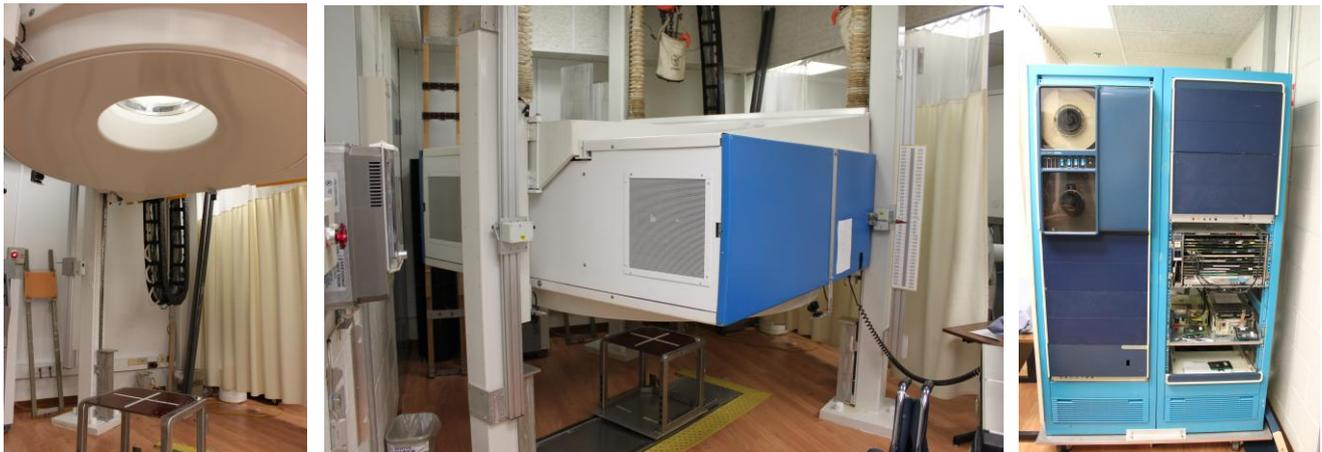
Fig. 12 Vertical axis XCT scanner installed at Fermilab. (L) Scanner in raised position. (C) Scanner in lowered position. (R) Scanner computer hardware.
