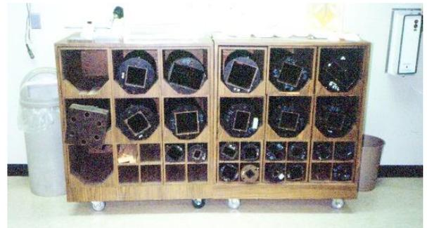
Fig. 23 (L) Single Benelex collimator cone at MDA. Length of collimator was 92 cm. (R) Cabinet with inventory of collimator cones for different field sizes.
