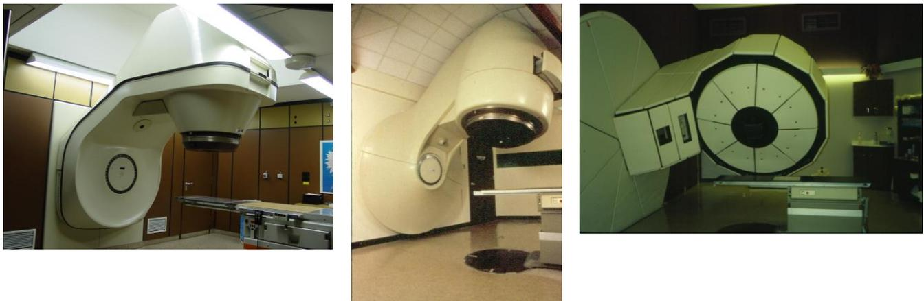
Fig. 13 Rotating gantries with approximately  $\pm 100^\circ$  rotation from the vertical. (L) Essen, Germany. (C) MDA. (R) UCLA.
