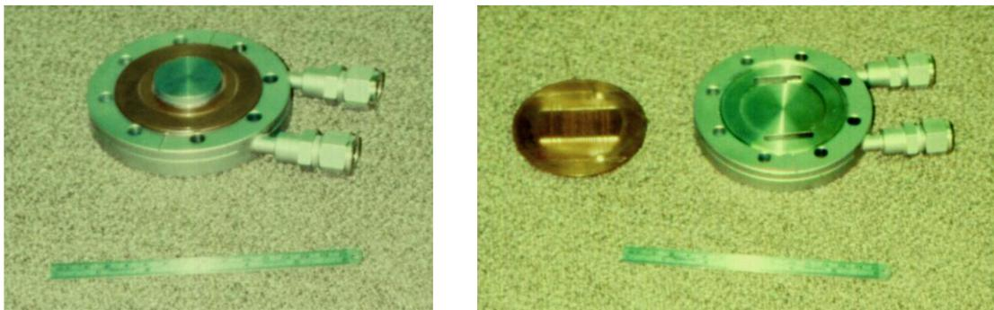
Fig. 19 Beryllium slab target and heat dissipation mechanism. (L) Surface at which the proton beam impinges on the beryllium. (R) Beryllium and copper slabs removed and turned upside down revealing narrow slits in the copper to increase the surface area over which water may flow for cooling.
