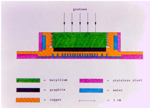
Fig. 20 UCLA neutron conversion target design. Reproduced from Moyers [12] that was modified from an original drawing by Miller (personal communication).
