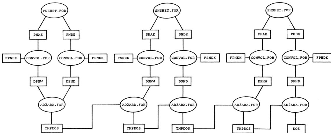
Fig. 29 Program flow for model that considered heterogeneous tissue and three radiation sources. Reproduced from Moyers [12].
