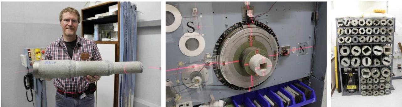
Fig. 25 Fixed cones used at Fermilab constructed of a mix of concrete and polyethylene. (L) Single cone held by Thomas Kroc. (C) Cone installed in radiation head. (R) Inventory of cones for different field sizes.
