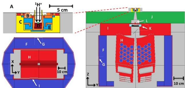
Fig. 4 Diagram of the UW CNTS target and MLC showing protons incident on the target (upper left), beam's-eye-view of the MLC (bottom left), and cross-sectional view of the beamline from target to MLC (right). (Reproduced from ref. 25.)
