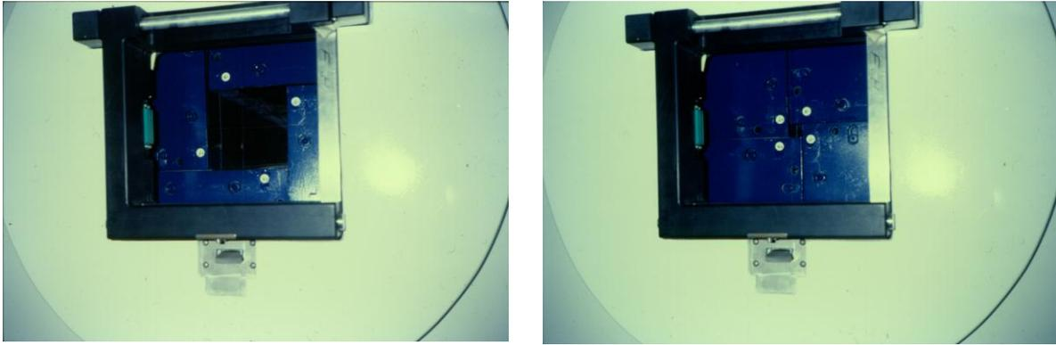
Fig. 26 Pictures of distal end of roman jaws type collimator installed at UCLA. (L) Opened to fullest extent that projects a neutron field with a size of 200 mm by 200 mm at the isocenter. (R) Closed to fullest extent that projects a neutron field with a size of 40 mm by 40 mm at the isocenter.
