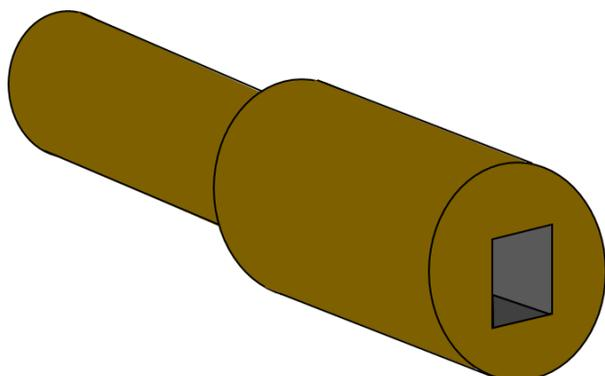
Fig 21. Schematic of the wooden aperture inserts used at Hammersmith Hospital. Similar apertures, constructed from various attenuating materials, were used in many of the early neutron therapy facilities
