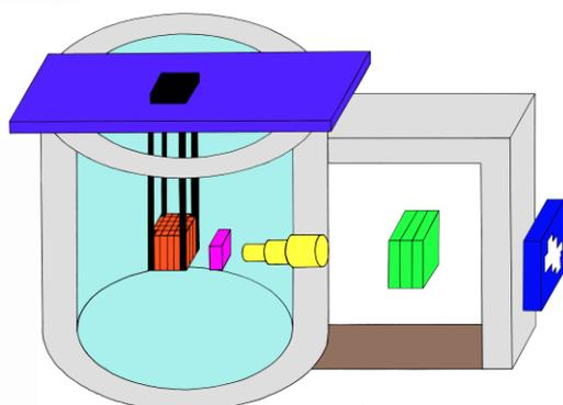
Fig. 1 Conceptual diagram of a research "swimming pool" nuclear reactor used for FNT showing the major components. Components by color: gray - shielding; red - reactor core; black - core support; aqua - water; purple - support crane platform; magenta - U-235 conversion target; yellow - fast neutron transport channel; green - beam filters; blue - MLC, brown: floor of equipment room.
