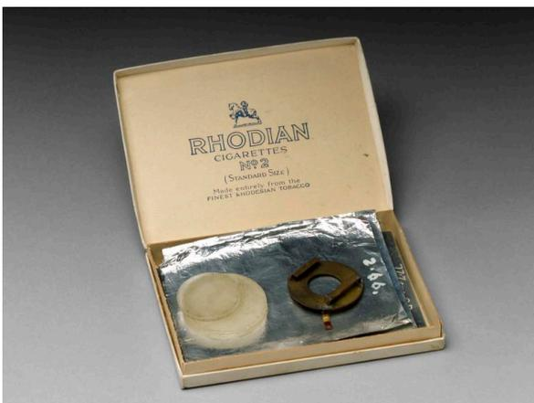
Fig. 4. Paraffin wax target, metal foils and foil holder which Chadwick used in his neutron experiments. This item is also on display in the London Science Museum
