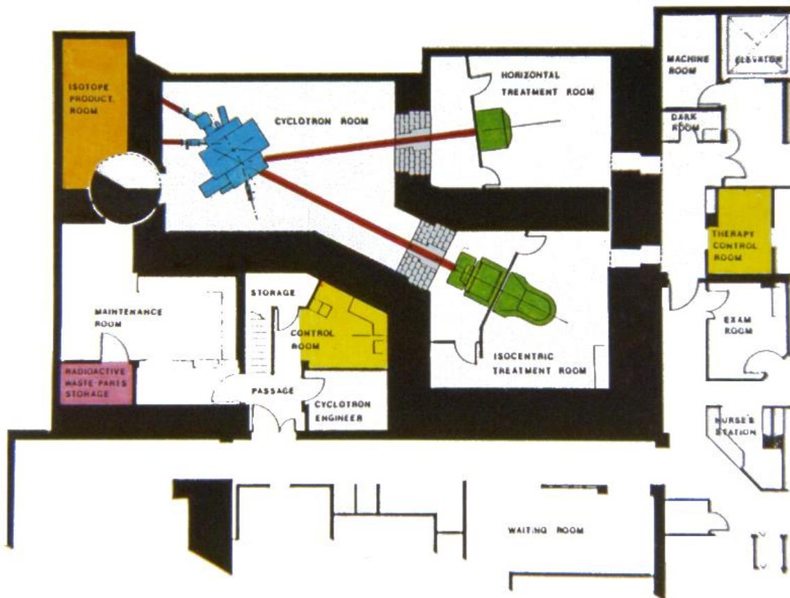
Fig. 5 Floorplan of dedicated medical cyclotron facility at MDA. One sliding shielding door was shared between the two FNT treatment rooms. One rotating shielding door allowed access from the cyclotron control room to either the cyclotron room or the isotope production room. Reproduced from Moyers [12].
