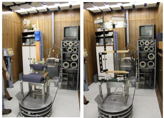
Fig. 11 Fermilab configurable patient positioner used in combination with horizontal beamline. (L) Configured for seated patients. (R) Configured for standing patients.
