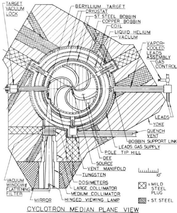
Fig. 9 Plan view of the superconducting cyclotron for FNT at WSU/KCC. (Image courtesy of the author.)
