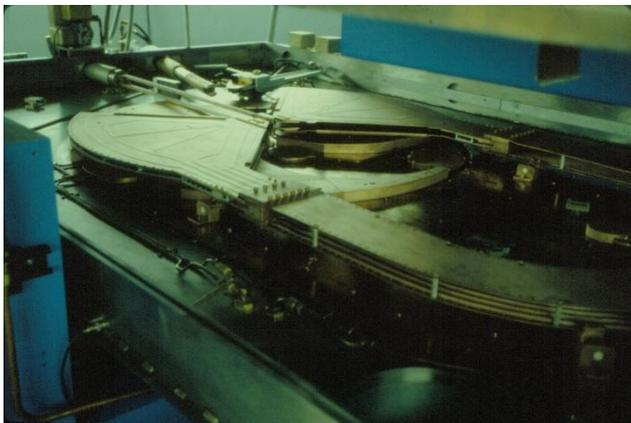
Fig. 6 Picture of inside of TCC cyclotron showing RF electrodes, pole tips, ion source, and beam diagnostics.
