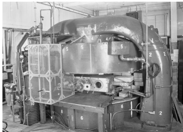
Fig 14. The 37-inch cyclotron used to treat the first patients with neutron radiation therapy. The magnet was the same one used for the 27-inch cyclotron.
