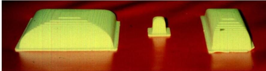
Fig. 24 Teflon flattening filters for different field sizes. The filters were inserted into the patient end of the collimator cones.
