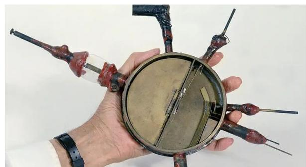
Fig. 6. Lawrence's original cyclotron fit in Glenn Seaborg's hand in this photograph.
