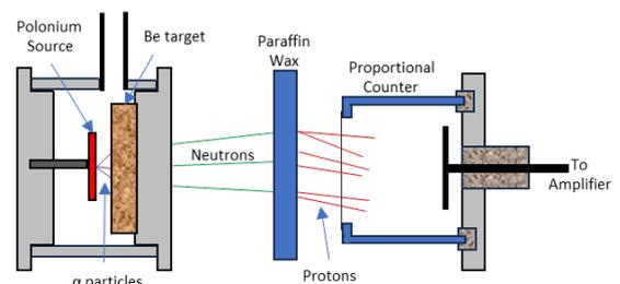
Fig 2. Schematic of Chadwick’s apparatus with which he detected the neutron.
