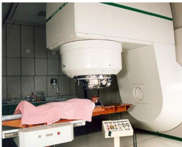
Fig. 6 Gantry and treatment couch for the iThemba fast neutron therapy facility. (Photo courtesy of Dan Jones.)
