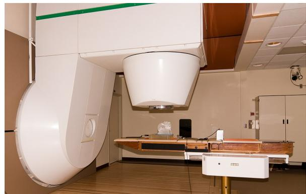
Fig. 3 Gantry and treatment couch for the University of Washington Clinical Neutron Therapy System (CNTS). (Reproduced from Wikipedia.)
