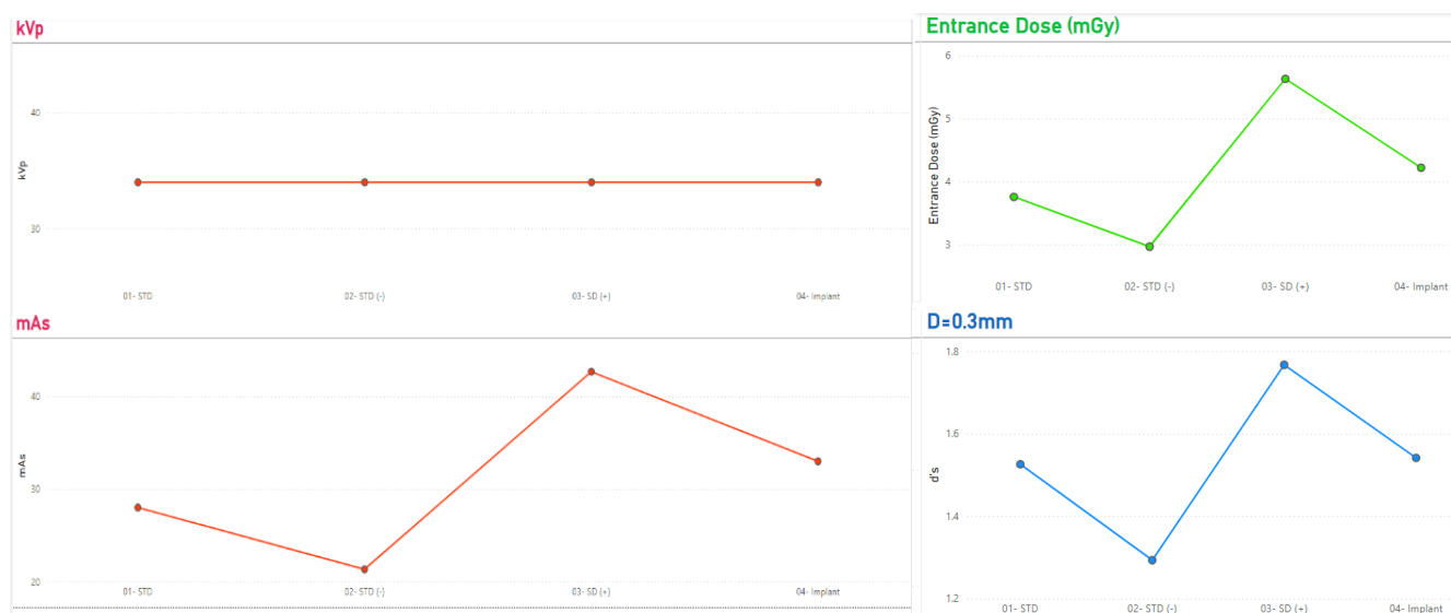
Figure 1: The average values of kV, mAs, detectability at 0.3 mm and Entrance dose (mGy) of three images taken under each of the three automatic protocols (STD-, STD+, and Implant) compared with the standard protocol of the mammography imaging equipment
