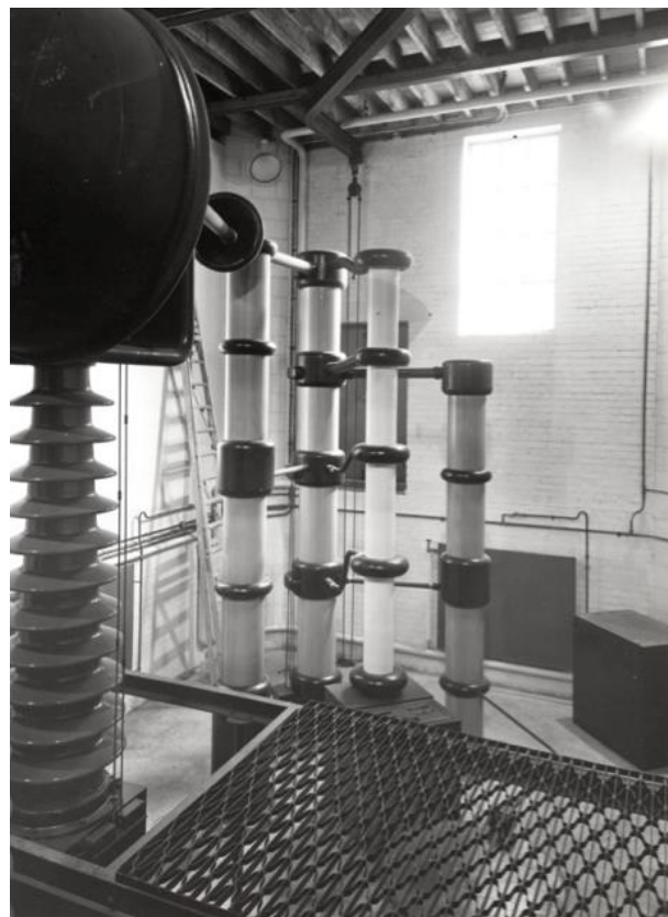
Fig 24. Photograph of one of the 500 kV Cockcroft generators. (Barts Health NHS Trust Archives)
