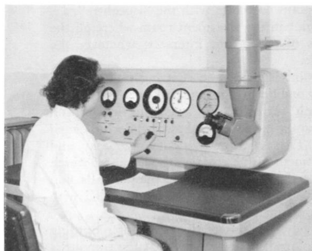
Fig 35. Control desk for 4MV linac with dose and dose rate meters; and periscope for patient viewing. Frank Farmer procured a cast-off submarine periscope for the Newcastle 4MV linear accelerator at Newcastle.
